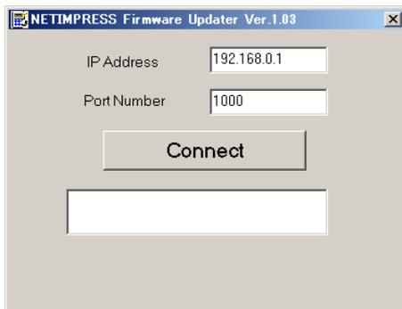
6. When the Ethernet communication is established, the current firmware version and the updated version are displayed. To update, please press the OK button.
