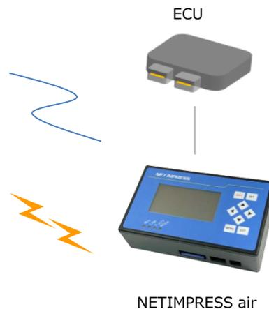
By adding each firmware (definition program file) for programming microcomputer into the SD card for NETIMPRESS air, it can support various devices.
