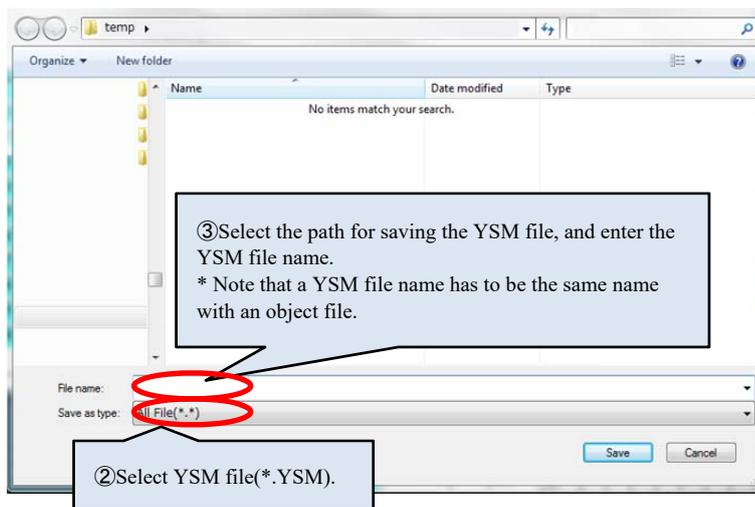
**✓** The SUM value check function which uses YSM file can also check the data in a certain area of buffer memory. You can also check the versions of the user object file by using this function.
