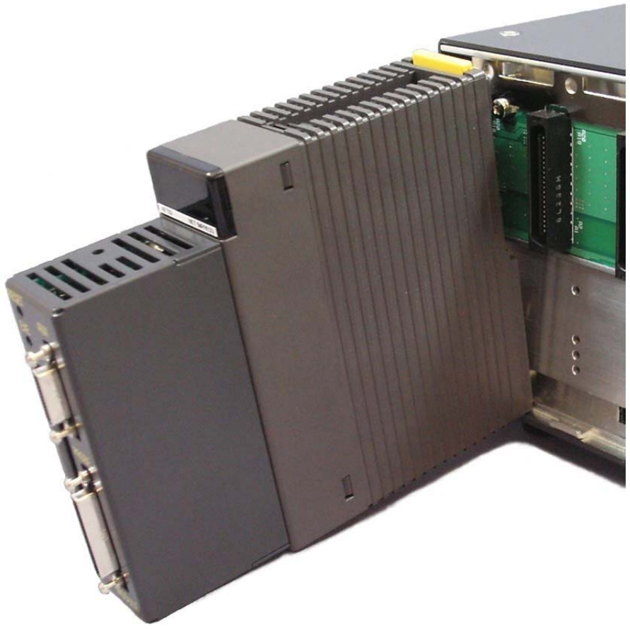
The Photo above shows that the concave portion of the programmer unit is hanged on the hook of the base unit (AF710).
