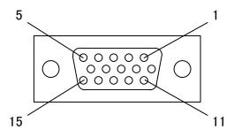
Connector pin arrangement (mate side view)
