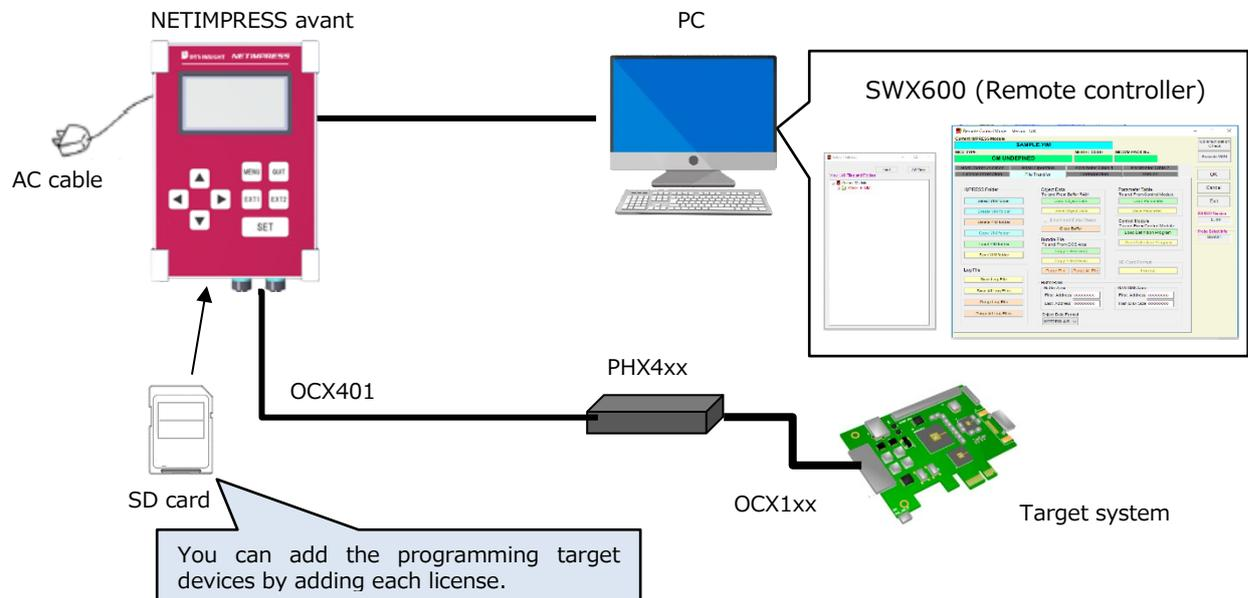
By adding each firm data (definition program file) for programming microcomputer into the SD card for NETIMPRESS avant, it can support various devices.
