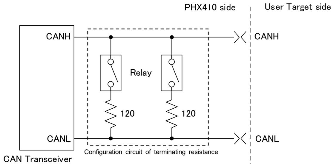
Relay's initial condition is "OFF" ("OPEN" condition: No terminating resistance).
